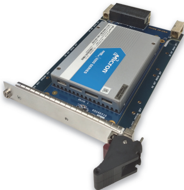
3U Open VPX Air-Cooled Module
