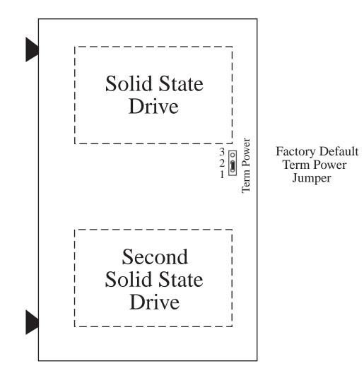
Figure 1-2: VX2-350-SC-SSD Jumper Configuration
