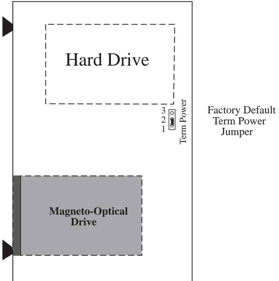
Figure 1-2: VX2-350-SC-DSMO Jumper Configuration
