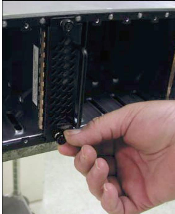
6. Go back to the top canister thumbscrew and thread it by hand until seated.
