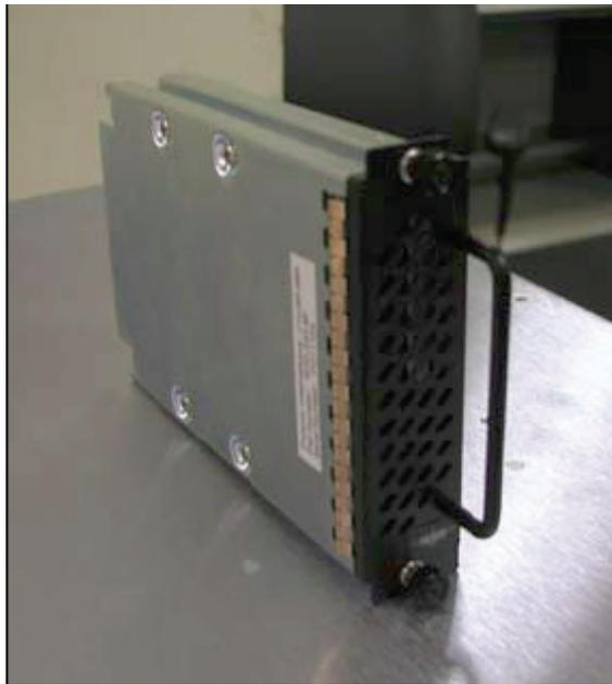
2. Holding the canister by the handle (**handle oriented to the right**) place it into
