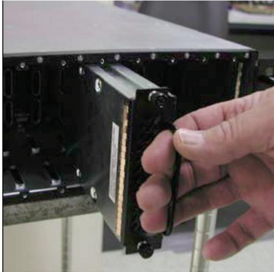
3. Slowly slide the canister all the way into the chassis until it bottoms out. A slight push on the handle or front of canister may be needed to fully mate the connectors.
