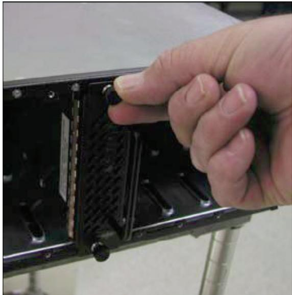
5. Thread the bottom canister
